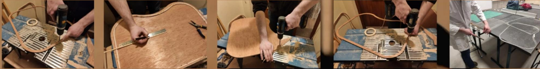
Cutting out top material to desired shape, prepping surface
