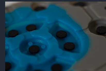
Buttons Carbon based pins in compression moulded silicon
