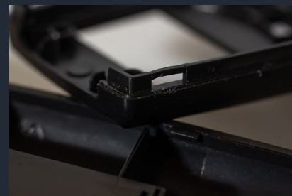
Semi-permanent snap hooks Broken snap-hook grooves from taking it apart
