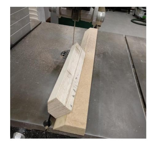
A 45\* jig was cut to allow me to make the cuts I needed to. They were also used to stabilize the pieces when cutting the mitres which I did not photograph
