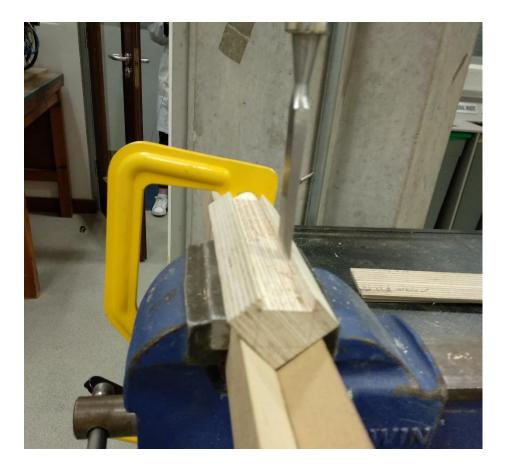
Once all my cuts were made, I had to chisel out the slot for the LED Rope light and the Perspex cover that I was going to fabricate as well. I also forgot to photograph the making of the Perspex
